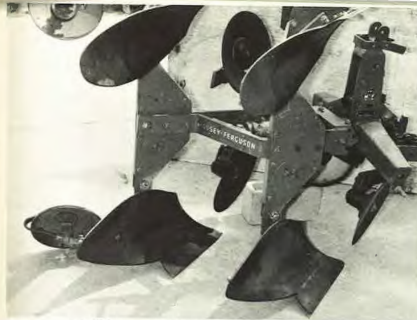
Figure 1. Reversible plow with concave disc coulters adapted to serve all bottoms while functioning.
