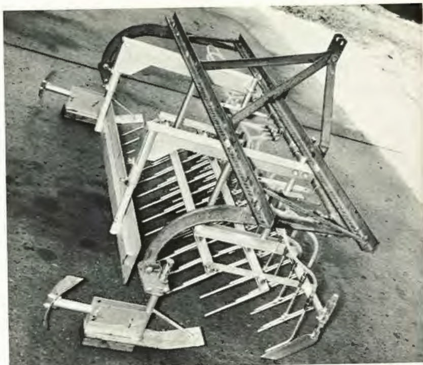
Figure 3. Combination tool for breaking clods, injecting herbicides and smoothing seedbed. Gage shoes mounted for depth control and wheel furrow scoring.
