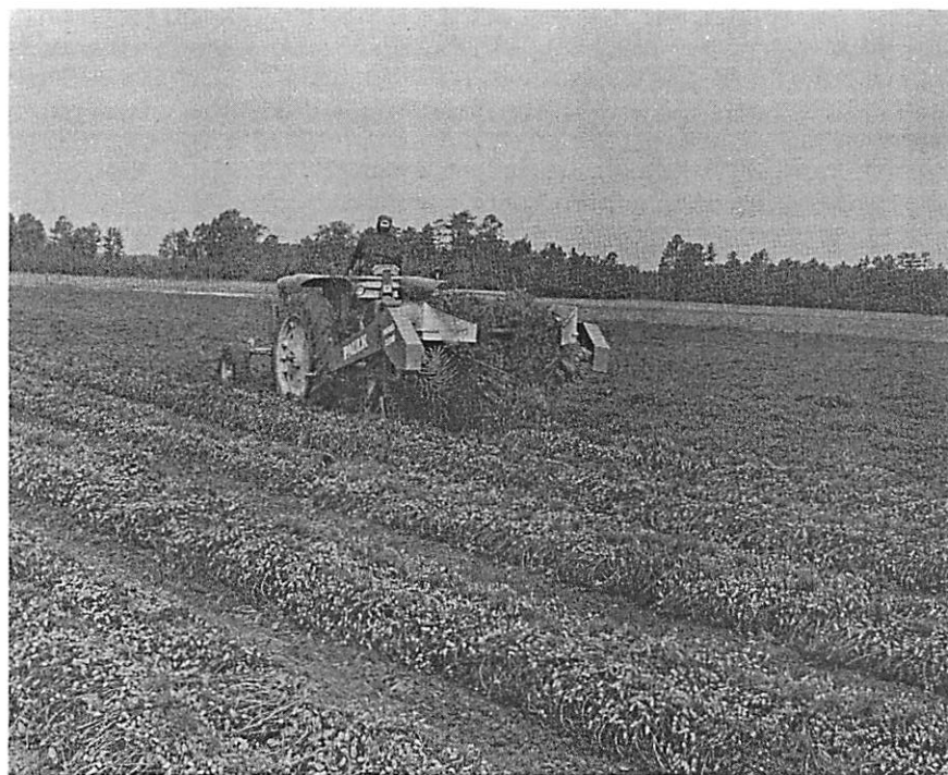
Fig. 2. Peanut digger-shaker-windrower producing an inverted windrow.
