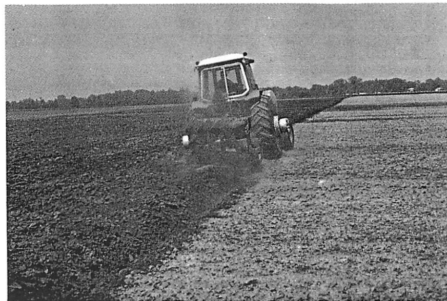
Fig. 2. Deep turning with a moldboard plow equipped with litter burial device is essential to achieving maximum yields in the SE.
